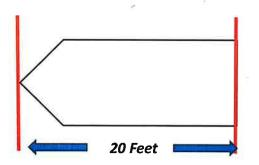
Measure speed boats from the tip of the bow/front to the end of the stern/back edge of the hull
